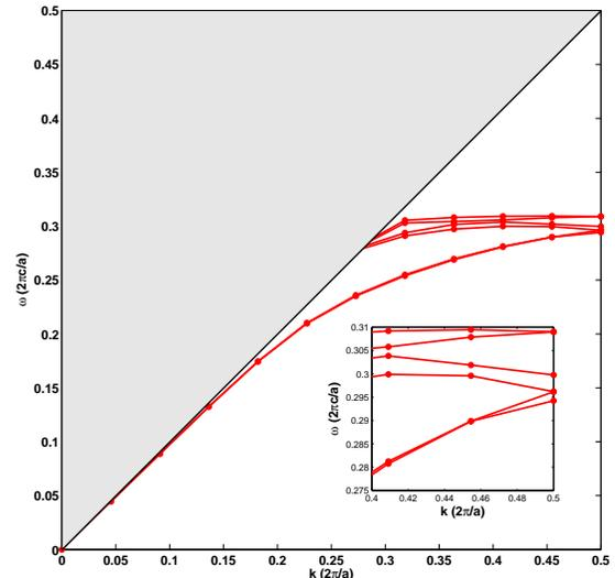
FIG. 6. Band structure of a 3-step spiral waveguide. The inset shows the bands near the zone boundary, where both 1-fold and 2-fold degeneracies are observed.
