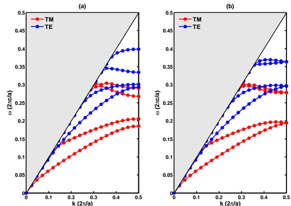
FIG. 2. (a) band diagram for the normal waveguide; (b) band diagram for the “shifted” waveguide.
